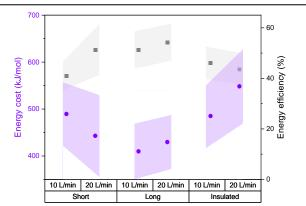
**Fig. 1**. Energy efficiency and energy cost metrics for CO<sub>2</sub> splitting using three types of C beds with GAP at SEI 3.7 (10 L/min) and 6.8 (20 L/min) kJ/L.
